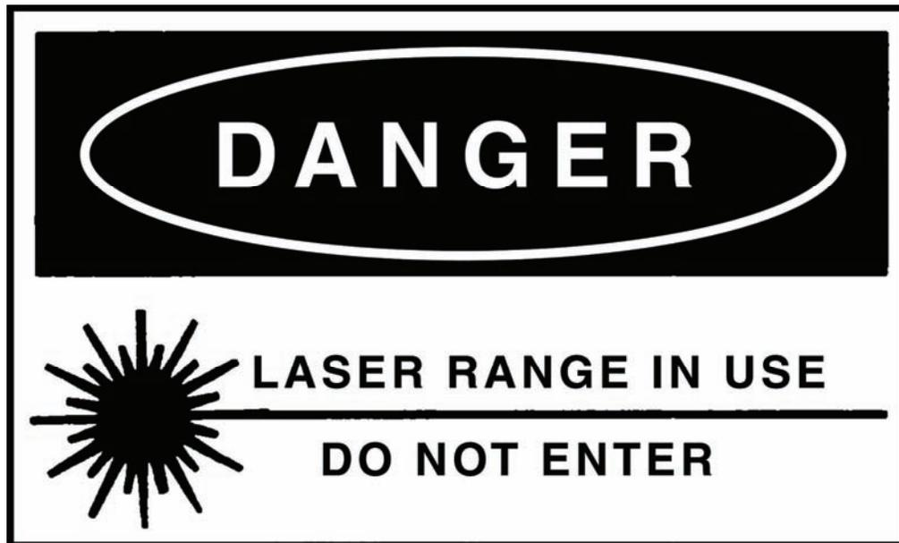
4-1. Class 3b and 4 Laser Controlled Area Warning Sign
